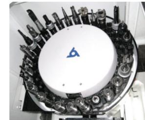
**Tool Handling** Efficient tool handling slashes idle time to maximize machining profit. The Mycenter-3020G ATC uses a memory-random tool selection system for smooth idle-free tool changes. Its generous 30 tool ATC enhances machining capability.
