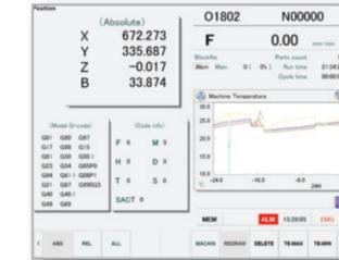
Our high efficiency **Intelligent Advanced Control System (IAC)** consists of a series of strategically located sensors and machine efficiency monitors that work to keep component growth due to machining heat build-up to less than ±5 microns (±0.0002").
